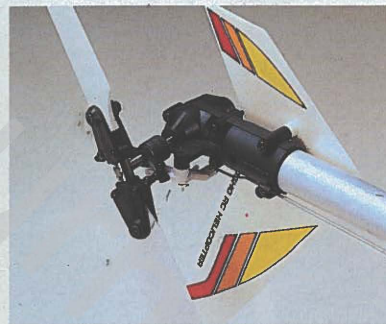
TAIL ROTOR SHAFT SUPPORTED IN BALL BEARINGS FOR SMOOTH ROTATION. PRECISE PITCH-CONTROL SYSTEM.
