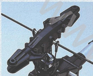
FLYBAR IS IN SAME PLANE AS MAIN ROTOR AND ACTS DIRECTLY, NOT THROUGH A LONG LINKAGE.
